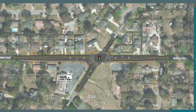
Scope: Improve the safety of the intersection at Fort Johnson Road and Secessionville Road with the installation of a traffic signal.
