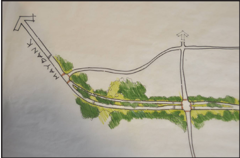
The TAP team recommended a hybrid three-lane approach for the Stono Bridge to River Road segment of Maybank Highway.
